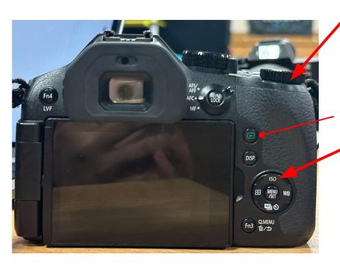
How to change Shutter Speed: Turn the button to the left and right without pressing any buttons
